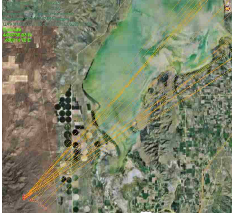
Figure 4.3: Visualization of the Hills Dataset. Locations of the readings are shown on the lower left side of the map and the bearings are represented by the lines. The icon on the top right side of the map approximates the known location of the transmitter (shown only for reference).
